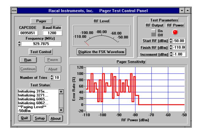
After creation of the test panel in the User Interface Editor, LabWindows/CVI was used to generate a "C" program shell that proved to interface the test panel to the pager test program. The rest of the code was produced using the LabWindows/CVI drivers along with some additional "C" code. A listing of this code is provided as an appendix to this application note.
