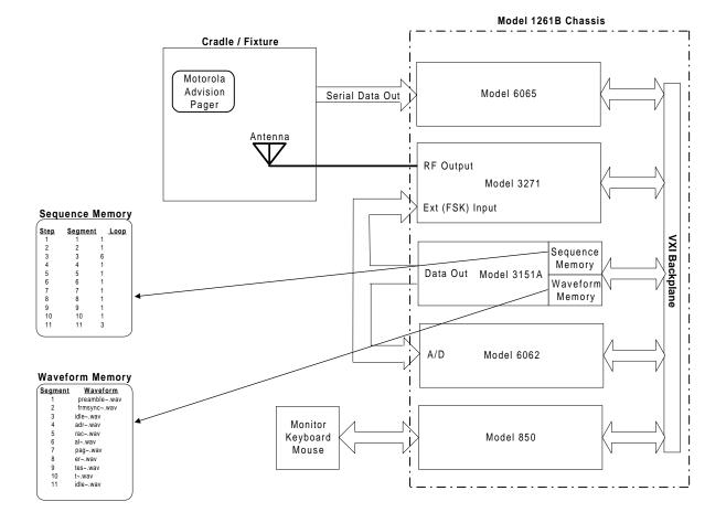
The equipment was then connected as in the following diagram:
